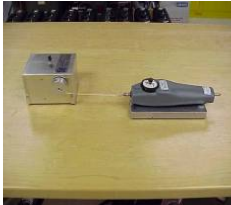
Horizontal Pull Slip Meter (HPS) Output = “slip index”
