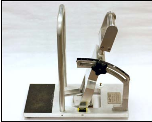
Brungraber Mark II (PIAST) Slip-Test Mark III Output = “slip resistance value”
