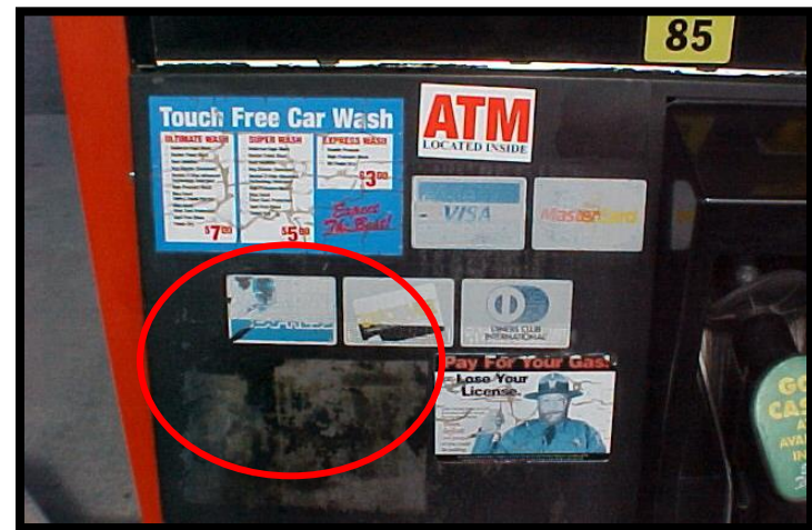
Torn, weathered or out-of date decals
