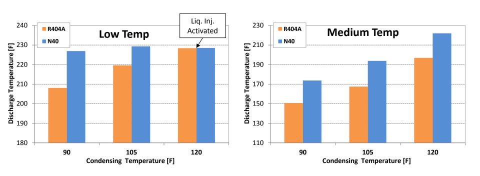
N40 Similar To R407A In Discharge Temperature Behavior Measured Test Results Confirm Theory
