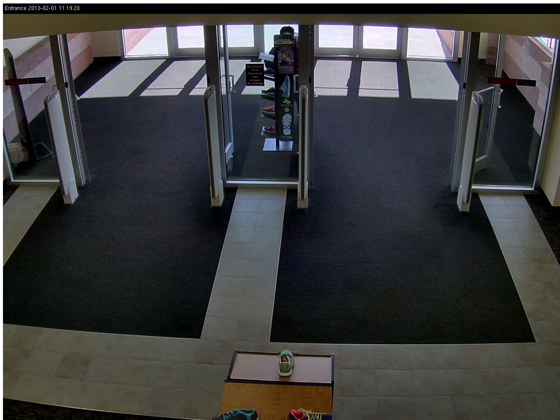
Figure 5: Image from a camera utilizing enhanced Wide Dynamic Range with Dynamic Capture for backlight compensation
