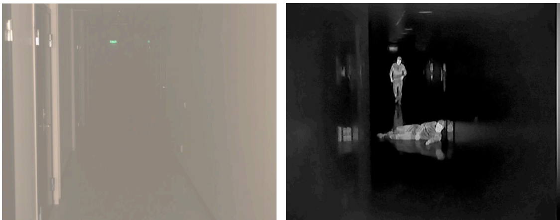
Figure 2: Image taken from a “regular” camera in a smoky hallway (left) and from a thermal network camera (right)
