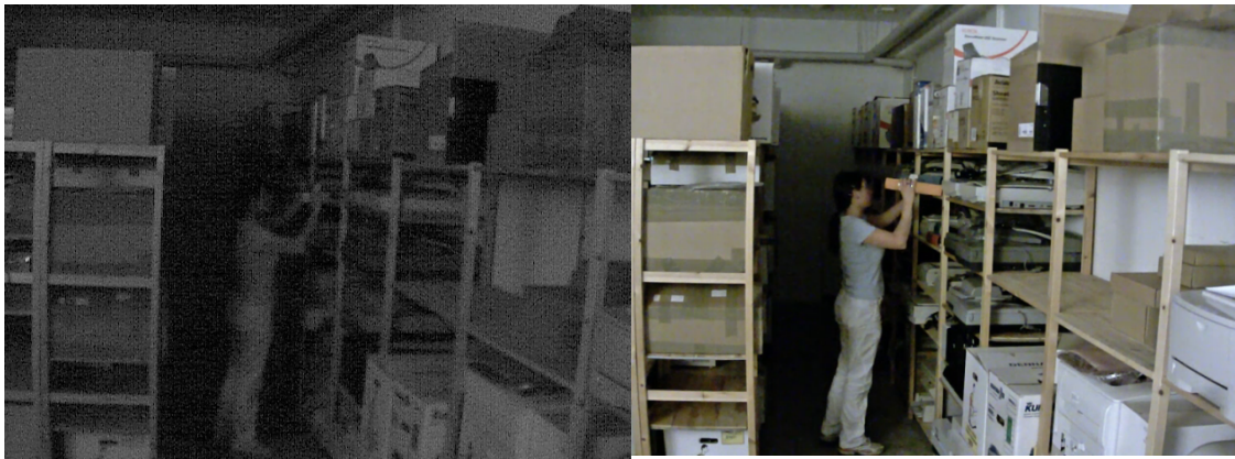
Figure 3: Comparison images showing a “regular” camera at 0.03 lux (left) and a camera utilizing advanced low light technology that finds the light in a scene for full color image (right)
